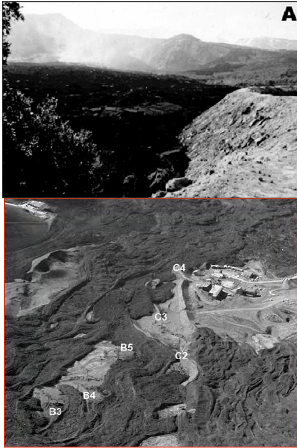
Figure 2. The control of lava flows. Earthen barriers orthogonal or transversal to the flow advancement direction. Left: 1991-92: lava advancement delayed for one month. Right: 2001: lava diverted toward less destructive paths.
